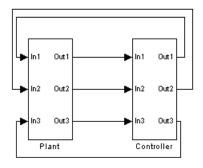
Your starting point in developing a plant/controller system is to model the system as two subsystems in closed-loop simulation. As your design progresses, you can use Simulink external mode with standard Real-Time Workshop targets (such as GRT or ERT) to help you model the control system separately from the plant.
